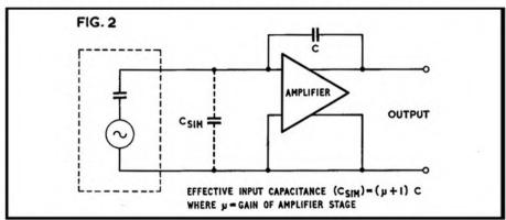
of the microphone artificially, by shunting it with a fixed capacitor—and in our example, a value of  $0.1\mu\text{F}$  will do nicely (fig. 1c). Now the total capacitance 'seen' by the input is ten times as high and 400K is optimum, with the response maintained down to 40Hz. This method has one great advantage: the signal-to-noise ratio is more easily preserved, since the combination is actually less susceptible to hum pick-up.
