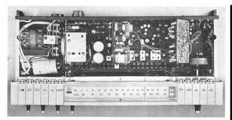
This is what you would see under the elegant case of a Beomaster 1000K F.M. Tuner Amplifier. Solid state circuitry throughout, separate and hinged component panels, stereo decoder already fitted, and components of the highest quality and closest tolerance.
