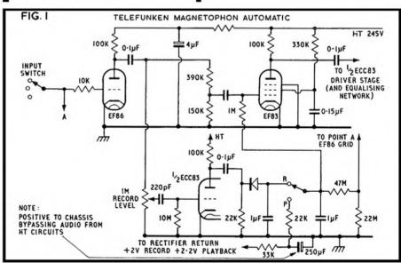
state, quite unequivocally, that this will never give as good results—as good hi-fi results, that is—as when normal control of recording is provided. There is, inevitably, some bass attenuation. But as the circuit is primarily intended for speech recording, interviewing and suchlike operations, this apparent drawback may prove all to the good.
