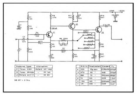
Fig. 5 Complete preamplifier circuit.
