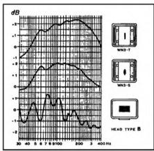
Close interval equalised low frequency response curves for differing pole constructions
