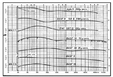
Fig. 7 Preamplifier response for given Standard Test Tapes from Miniflux Type WN3-T and WN3-S heads.
