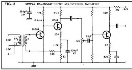
amplifier. The circuit has been somewhat experimental in nature, but the results are quite reasonable within the limits set by economy, and one amplifier to this design has been in the mixer now for a while; no performance measurements have been made, but when used with an inexpensive moving-coil microphone the emerging sound is quite reasonable, which was after all the basis of the design philosophy for this amplifier.
