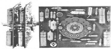
Tape preamplifier mounted on Miniflux printed circuit board.
