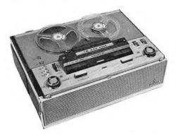
0.08% RMS.  $3\frac{3}{4}$  i/s speed imperfections were almost equally satisfactory at 0.1% RMS, and top and bottom limits of 0.09% and 0.11% RMS (see fig. 1). At the lowest speed of  $1\frac{7}{4}$  i/s, readings averaged 0.15%, with a just audible cyclical speed variation at approximately four per second.
