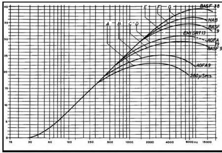
Fig. 1 Unequalised output from Standard Test Tapes.
