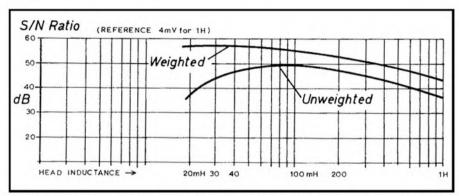
Fig. 4 Signal to noise ratio of germanium transistor input stage for differing head inductance values.
