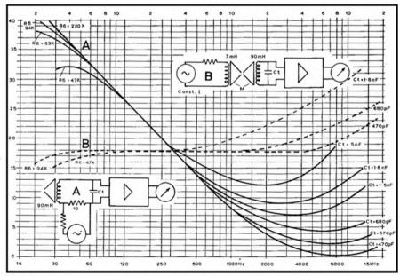
Fig. 6 Preamplifier response curves from constant voltage generator including head tuning.
