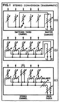
(a) Simplest conversion, with one amplifier switched to right or left channel, and ganged mixing stages.
