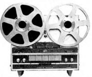
A studio type 3-speed 4 track stereo/mono recorder of professional quality. Fully solid state, 20 watts per channel amplifier; Crossfield heads; 10½in. reels; keyboard controls, and many other features. 190 gms. Interest Free Terms. Deposit £66.10.0 and 12 monthly payments of
