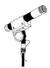
Completely cordless, all contained in one neat unit, no bigger, no heavier than a torch, no following flex, no bulging pocket transmitter. This exclusive integrated Microphone Transmitter includes a microphone capsule complete with Cavity, Transmitter Unit and Rechargeable Power Supply. The Hike-Mike is available for single or multi-channel operation with existing systems and embodies SHURE microphone inserts to provide studio quality performance. Patent applied for.
