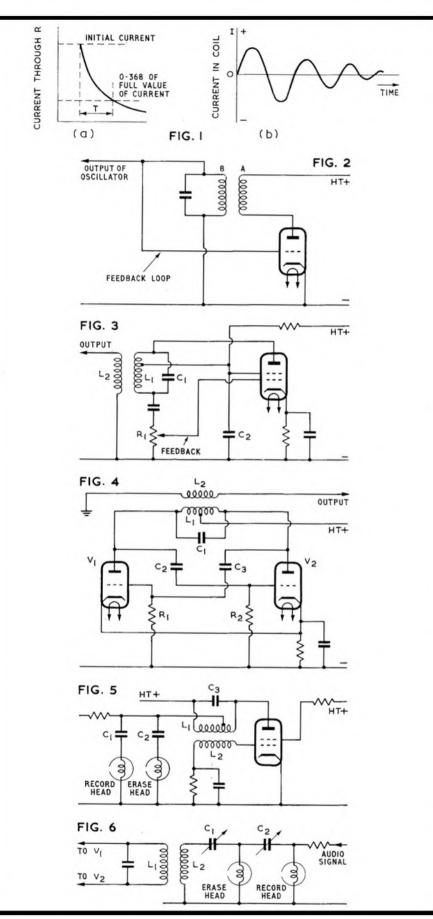
tortion in the bias waveform shows up as noise. Moreover, the greater the demand upon the oscillator to provide enough current for adequate erasure, the greater the likelihood of distortion. The push-pull circuit therefore scores over most single-ended oscillators because of its lower distortion for the same output.
