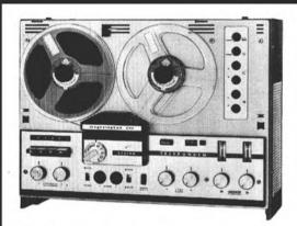
**TELEFUNKEN 204E Stereo.** Special multiple-function switch controls six different functions, gives greater operating convenience and flexibility of control. Mono and stereo—four track recording/playback, frequency response at  $7\frac{1}{2}$  i.p.s., 40-18,000 c.p.s. Two built-in speakers, 6 watts per channel output. Save 20 gns! List price 106 gns., our price 86 gns. or on interest free terms £22.12.0 deposit and 12 monthly payments of £5.12.10.
