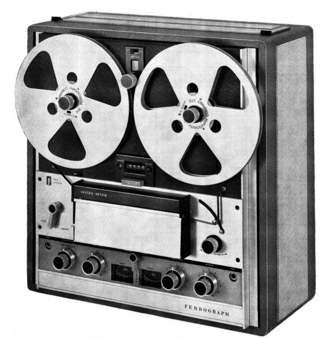
**21.** 2 inputs per channel with independent mixing (ability to mix 4 inputs into one channel on stereo machine).
