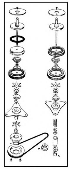
Fig. 6. Exploded view of Akai clutch.
