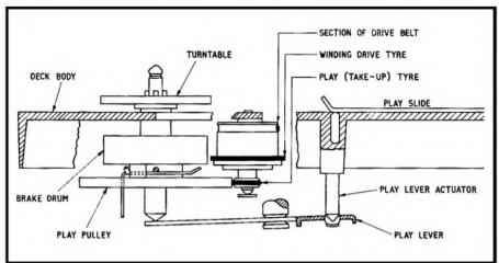
Fig. 8. Ampex 753 arrangement.
