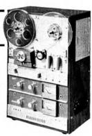
AKAI 3000D 4-Track Stereo Tape Deck (above). High Quality Three Heads System. 4-track stereo/monaural recording and playback. For playback, the 3000D requires external power amplifier and speakers. 2-speeds (32 and 71 ips). Three heads (erase, recording and playback heads). All silicon transistor pre-amplifier. Automatic shut off, Pause lever. Tape cleaner. DIN jack. Stereo headphone jack, 3-digit index counter with reset button. VU meters. Beautifully grained wooden cabinet. £99 10s.
