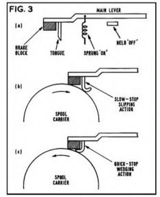
beginning of a fast wind is enough to spill off tape from a badly braked spool.
