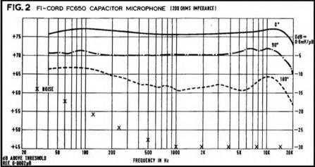
an output of 5 mV for a 26 mm diameter unit. The lowered sensitivity of the microphones under test is proportional to the drop in voltage to 65 V but this is inevitable with the relatively soft plastic diaphragms used in these microphones which would be pulled against the back plate by a higher polarising voltage.
