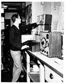
A corner of the BBC Radiophonics Workshop. The audio signal generators are coupled to a keyboard system providing varying degrees of attack and decay.
