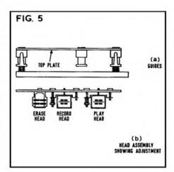
head is replaced, the only way of making sure is to experiment with shims between the head and mounting plate. Record/play heads have more scope for screw adjustment.
