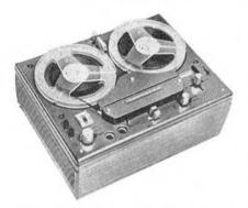
MANUFACTURER'S SPECIFICATION (19 cm/s). Quarter-track transistor stereo tape recorder with cross-field bias, power amplifiers and side-facing monitor speakers. Wow and flutter: 0.1% RMS. Frequency response: 40. Hz - 18 kHz ±2 dB. (In amplifier mode 30 Hz-16 kHz ±3 dB.) Signal-to-noise ratio: 55 dB ref. peak recording level. Spool Capacity: 18 cm. Tape speeds: 19, 9.5 and 4.75 cm/s. Modulation indicators: Meters. Sockets: Three pin DIN (*microphone*), five pin DIN (*line*
