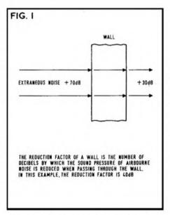
*factor*, which is the number of decibels by which the sound pressure is reduced in the process of passing through the partition (fig. 1).
