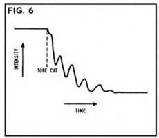
ation times are associated with large studios used for orchestral music. The reverberation causing the individual sounds to 'blend' together. For a studio where a variety of sounds are to be encountered, a short natural reverberation time is required, longer times being obtained when necessary by the use of artificial reverberation.
