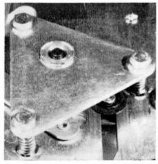
bolts are used to adjust both the overall height and the verticality. The spools should sit 3 mm clear of the top cover, and should, of course, be level with the main deck and with each other. A ruler held across the faces of the two spools while they are slowly rotated shows up any tilt. Take a bit of trouble with this adjustment; so much depends on it.
