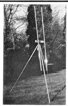
chromed towel rail brackets. The tripod proved stable over a wide range of boom positions, two-thirds forwards plus the weight of two fairly heavy ribbon or dynamic microphones causing no excessive imbalance.
