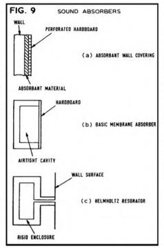
vided by *membrane absorbers*, which consist of a panel of non-porous material such as hardboard covering an airtight cavity (**fig. 9b**). The hardboard acts rather like a drumskin, having a fairly low resonant frequency at which it is a very efficient absorber.
