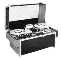
Three Bell & Howell models were submitted for evaluation, one incorporating editing facilities and another in prototype stage. The analysis was of monochrome performance though all three VTRs were capable of PAL colour, convertible instantly to any other system by the addition of a plug-in circuit board. A major fact in favour of the Bell & Howell models was their tape consumption, 30% lower than competing designs.
