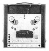
The Belgian Carad R.59 (illustrated) possessed the extraordinary feature of slide-axis spool turntables which could be set to accommodate 18 cm spools without overlapping the cabinet, or swung out to increase the spool capacity. A  $\frac{1}{2}$ -track stereo recorder, the R.59 operates at 19 and 9.5 cm/s. In its cheapest unit form, it sells in France for £175.
