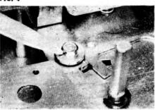
The bolt indicated in this view is that under which the interlock lever slides, and we must check that this is clear of swarf, etc, and apply a thin smear of grease to help the action.
