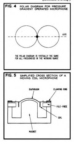
the source off the axis of such a microphone, the HF may be reduced whilst retaining the same LF content as would be obtained if the source were positioned directly in front of the microphone.
