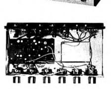
THIS is a nicely styled, self-powered sixchannel mixer for three high impedance microphones, two low-level 600 ohm inputs, and an equalised phono input for either magnetic or ceramic pick ups.
