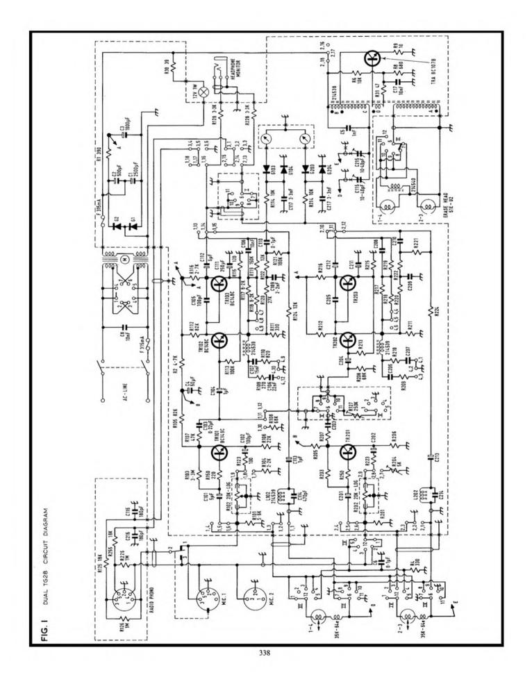
and the shielding of the heads much improved compared with the earlier TG27, so that the hum bucking coils are not called upon to do an impossible task but only to reduce the slight hum almost to vanishing level.
