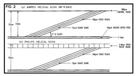
Ampex single-head helical scan using 25 mm tape gives a trace speed 2200 cm/s, increasing to 25,400 cm/s on 60 Hz mains.
