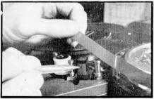
C Crossed belt drive and electromagnetic brake.
