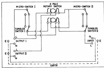
Key diagram to the wiring of the complete unit.
