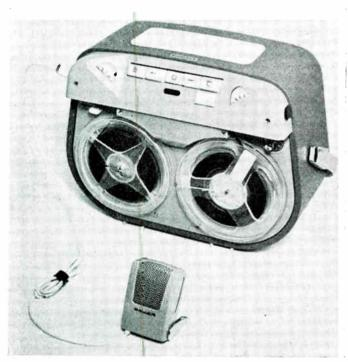
This view of the Butoba shows the sloping control panel with its row of push buttons and the flanking tone and volume controls. Just above the 5 in. spools can be seen the speed change lever (left), and the clock type position indicator. The bar type magic eye is centrally positioned just below the off button.
