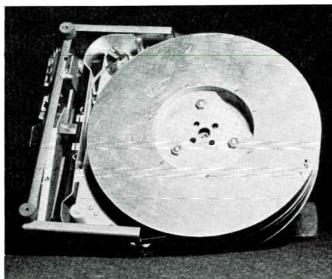
All together 20 hours of material are stored on a single cassette. The head (centre left) can be selected to scan any one of the 18 tracks. The push-button selector trips the spring-loaded head carriage once on each depression (see lower photograph).
