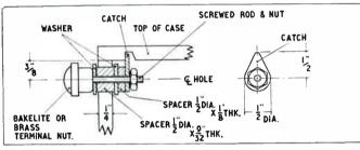
Detail of the door catch, made from a radio terminal.
