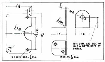
Micro-switch mounting plate (left) and rotary switch bracket.
