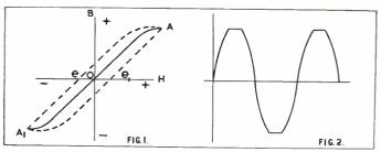
Fig. 1: Showing the straight part of the curve A<sub>1</sub>OA traversed by the audio signal; and Fig. 2: the effect of overloading.
