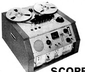
The 1151 illustrated is shown fitted with an operational panel designed for broadcast studio use.
