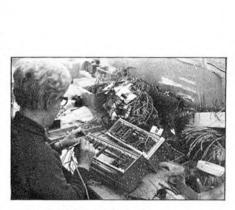
Fig. 4. Wiring circuit boards.
