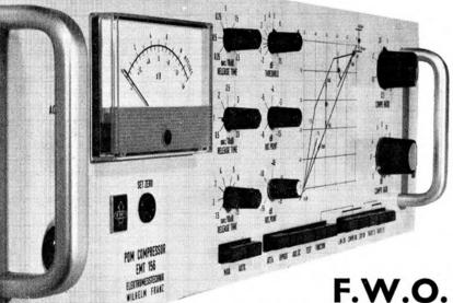
**OPERATES AS COMPRESSOR** LIMITER OR BOTH; AVOIDS NOISE **INCREASE IN PAUSES BY EXPANDING** AT LOW LEVELS.
