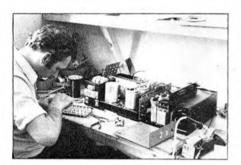
Fig. 7. Assembly of tape tension servos.
