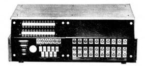
The Neve BCM 10/2 marks a new departure into the field of sophisticated audio control. It embodies ten full mixing input channels and two output groups and is conveniently transportable.
