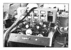
Fig. 9. 8-track 25.4 mm recorder partially assembled.
