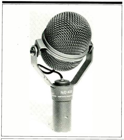
hese dynamic microphones are just two from a range introduced by Electro-Voice within the last year under the label of the N/Dym series. They take their name from the use of a Neodymium alloy used within the magnet structure of the mics which Electro-Voice claim gives the mics' magnets four times the power of conventional microphone magnets. Further, the design offers increased sensitivity and a more uniform magnetic field, which E-V say lowers distortion during peak sound pressure levels.
