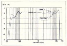
Fig.1: Record to replay frequency response. Channel 1 Dolby, channel 6 non-Dolby. Referenced to -10 dBu input
