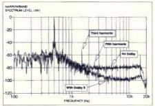
Fig.3: FFT spectrum of 500 Hz (record to replay). Input level -10 dBu. Channel 1 with Dolby *S*, channel 5 without
