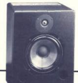
Q108 - 2 way active system with twin integral 100W power amplifiers and high quality BSS crossover network. 8" bass driver/1" soft dome ferrofluid cooled tweeter.
