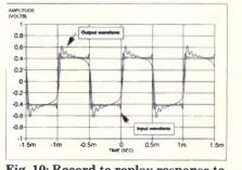
Fig. 10: Record to replay response to 1 kHz square wave. Channel 1 input level -10 dBu. With and without Dolby S
