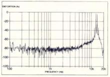
Fig. 7: FFT spectrum of channel 1/3 and 14 kHz 1:1 CCIF tone (record to replay). Input level 0 dBu. Ch. 3 with Dolby S
