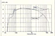
Fig.2: Record to replay frequency response. Channel 1 Dolby, channel 6 non-Dolby. Level referenced to 0 dBu. Note drop off of non-Dolby signal at higher input level
