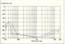
Fig. 8: Record to replay crosstalk (dB). Channels 2/3 recorded, channels 1/4 measured — both very similar. Input level to channel 2/3 = -10 dBu with noise reduction
