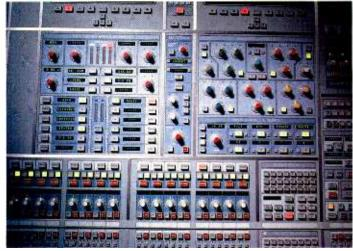
Close up of area of control surface covering EQ, dynamics, channel flow and multitrack
