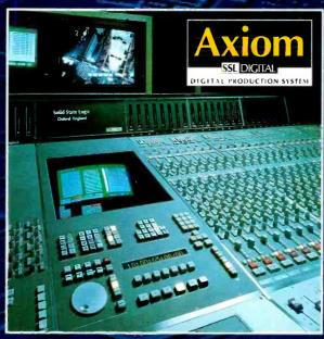
Fully digital, fully automated/resetable production console. Axiom is a single system with integrated multitrack recording, non-destructive drop-ins, editing, sequencing and playback, all with the same high audio quality
