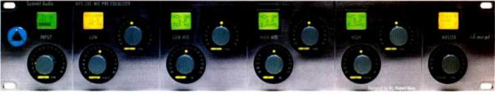
controls Channel mode (dual or stereo), Channel Select (for adjusting settings) and locking of presets. Any changes made to a locked preset are lost when changing to another preset. The screen also enables the Fader screen. The Output Fader (dark green screen) allows complete fades to be made to either the A or B channels or both together. In normal operation, the Fader function is disabled.
