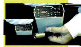
table digital and analogue output levels, plus channel ident on CH-B digital and right channel analogue. Validity bit selection for audio/data identification is also provided. LM1 monitor supports the same sample rates and has a headphone output with volume control. Accurate level indication is given for digital and analogue inputs, plus digital status and error monitoring.
