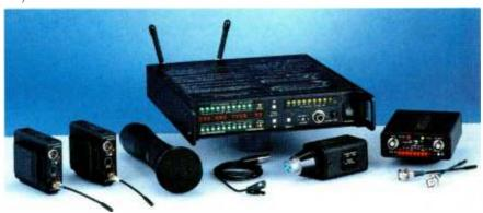
untouched while low-frequency distortion will be present. The converse is true for a time constant set too slow. To eliminate this, the Lectro has dual-band companding; two separate companders fed from a crossover network that separates the frequency bands at 1kHz with a 6dB octave slope.
