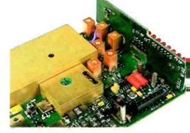
Two small green LEDs marked 0 and 180 show the phase difference between the signals being received at the two antennas.
