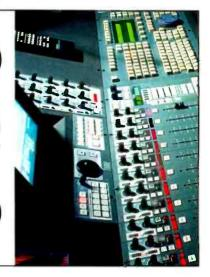
Mixing. Fully integrated digital mixing to 5.1 surround with dynamic automation, snapshot recall, virtual effects and up to 48 motorized faders.
