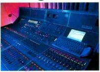
he Digital T Series console combines the assignable control surface of the established T Series mixing system with an alldigital signal path. Aimed at on-air and production applications, the system is designed to provide the same level of reliability as the existing T Series. In the event of failure, control panels and DSP cards are designed to be hot-pluggable, so that they can be swapped while the rest of the console is still in operation.
