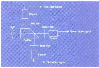
Fig.1: Simple colour television system. Camera image is split by three filters. Red, green and blue video signals are sent to three primary coloured displays whose images are combined
