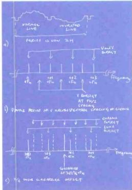
Fig.4: PAL spectrum and origin of subcarrier frequency. See text for details
