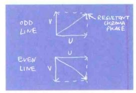
Fig.3: In PAL, phase of V signal is inverted every other line
