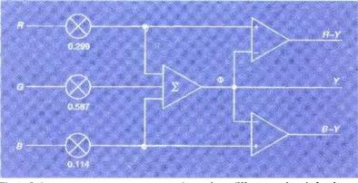
Fig.2: Colour components are converted to colour difference signals by the transcoding shown here
