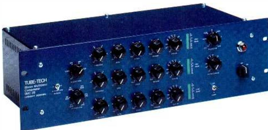
The TUBE-TECH SMC 2B is an all tube based stereo multiband opto compressor. It features variable x-over frequencies between the three bands. Each band features separate ratio, threshold, attack, release and gaincontrol. A master balance and output gain controls the overall level.
