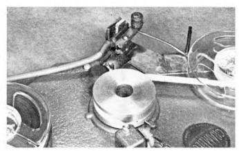
The photograph shows the Gramdeck fitted with the pneumatic pause control designed by the author.
