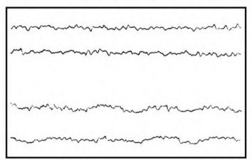
Fig. 4A Top two fluttergrams readings at 7½ i/s, 0.1% R.M.S. Fig. 4B (lower pair) 3¼ i/s, 0.15% R.M.S.
