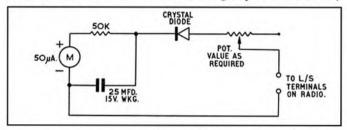
be required. Any standard crystal diode may be used. If you need to increase the sensitivity of the circuit, any loudspeaker output transformer can be used, connecting the low (3 to 5 ohm) side to the set, so that if functions as a step-up transformer.
