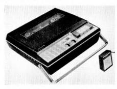
Quarter-track stereo recording facilities are included on the MR.151, which has speeds of  $3\frac{3}{4}$ ,  $1\frac{7}{8}$  and  $\frac{18}{8}$  i/s and takes 5in. spools. Output power is quoted as 0.9W per channel through internal side-facing speakers. Pause control and twin VU-meters are incorporated. This model operates from six U2-size cells or mains and has a 35dB signal-to-noise ratio. Price has yet to be decided.
