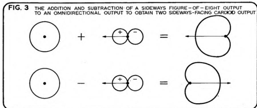
the sides (as microphones A and B have no response at the sides), and no response at the front or back (due to the subtraction of outputs), but a fair response in all directions at 45° from the front or back, as illustrated in fig. 6. Because of the shape of its directional characteristic, a microphone whose sound pick-up (polar response) is as in fig. 6 is called a *clover-leaf* microphone.
