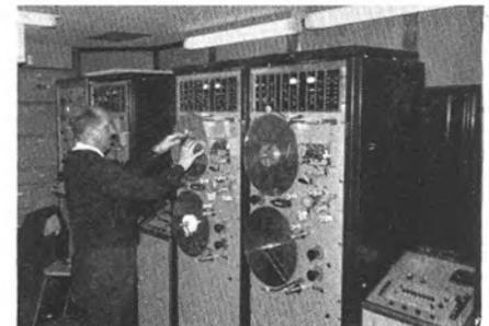
line, a Westrex compressor used to keep the dynamic range within reasonable limits, levels being controlled on a four-channel Vortexion mixer. The main recording was made on a Gaumont Kalee 16 mm edge track machine and backed at 19 cm/s on a TRD recorder. A further recording was made on a Grundig *Stenorette* for transcription purposes. In the speech cubicle are a telephone, a ribbon microphone for the 'rear' voice, and a GPO telephone matching unit.
