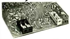
Half the size of Bantam Jacks, the new PCB Jacks are only 1.25" long, 0.435" high and 0.365" wide. Mount directly on PC Boards wherever access is required. Normal through-jack configuration allows
