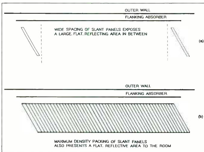
**FIG 4: Effects of extremes of slant panel spacing**
