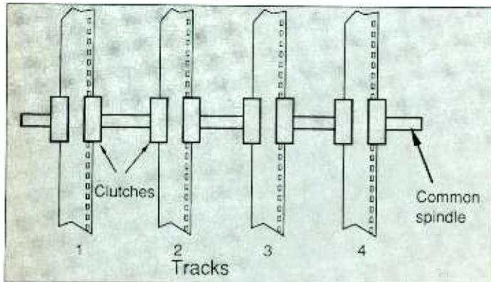
FIG 1: On a flatbed film editor tracks are locked mechanically, but may be 'slipped' with relation to each other by means of clutches
