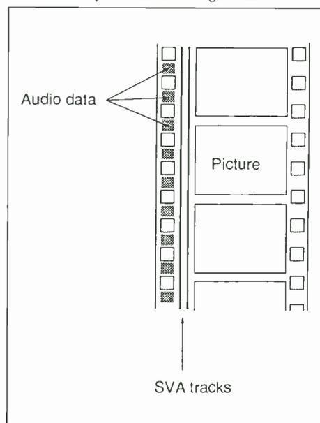
FIG 5: Dolby *SR-D* places optically recorded digital audio data patterns in between sprocket holes, leaving the SVA tracks of 35 mm Dolby *Stereo* intact
