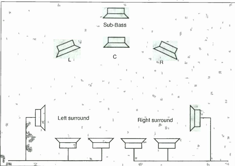
FIG 4: Six sound channels are involved in the SMPTE recommendations for digital film sound formats, as shown. Sub-bass is limited to <100 Hz
