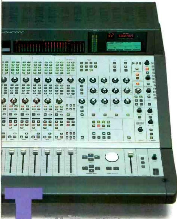
**T**alk about perfect timing. As audio is increasingly generated, edited, processed and recorded in the digital domain, along comes Yamaha with the DMC1000 – an all digital production/recording console with 22 inputs, 10 busses and 4 auxiliary busses, capable of handling all the major digital formats.
