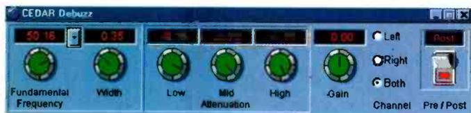
So along comes Debuzz. This is a totally new process in concept and operation, and for the time being forms part of the CEDAR for Windows collection, running on a PC with the CEDAR ProDSP hardware installed to provide the powerful processing capabilities it needs.
