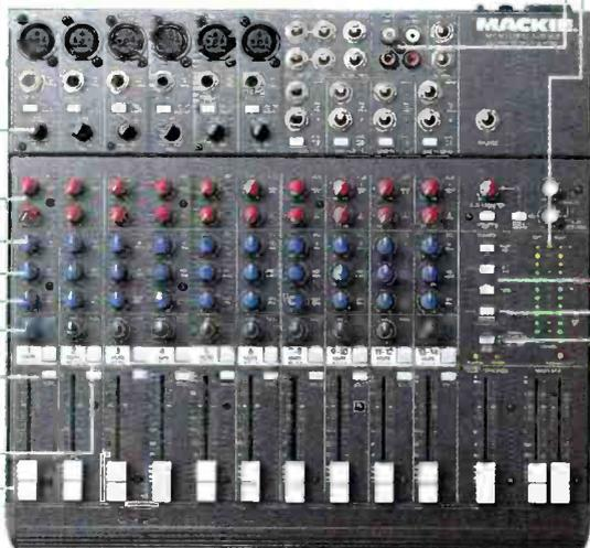
All inputs & outputs are balanced<sup>1</sup> to cut hum & allow extra-long cable runs, but can also be used with unbalanced electronics. <sup>1</sup>except RCA tape jacks, headphone jack & inserts.
