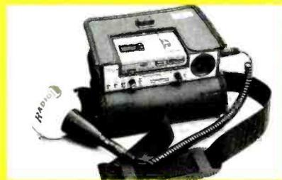
a 1/4-inch jack headphone socket. A recording level control with LED PPM and a monitor volume control are located on the front panel. It is powered by internal Ni-MH rechargeable batteries. The Carrier is a simpler and cheaper version of the MobiDisc and is similarly built around an MZ-R30 machine. It features a mono (or stereo) XLR mic input, a stereo cinch line output and a 1/4-inch stereo jack headphone output.
