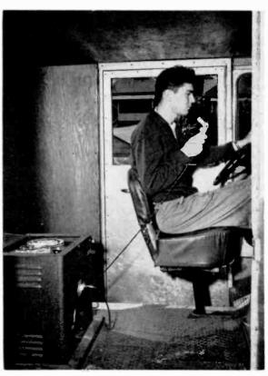
Most commercial sound trucks used in political campaigning today have switched to tape since rough roads offer no problem. This unit is in a sound truck used by a Minneapolis firm and uses a Carter motor generator to provide the necessary AC current for the tape machine.
