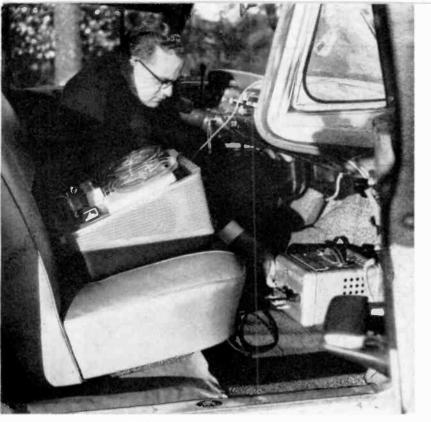
Here an ATR inverter mounted on the floor of a campaign station wagon is shown together with a Bell & Howell tape recorder used for a wide variety of purposes. Incidentally, the inverter provides a handy plug-in for electric razors to help keep the candidates in tip-top appearance.
