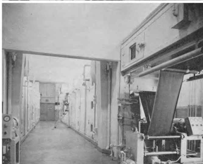
Upper left: loading the rolls of raw backing stock in the coating machine at Audio Devices. The raw stock is carefully protected against contamination from the time it leaves the machine which makes it to the finished tape. Upper right: a Uni-level coating machine at the Reeves Soundcraft plant. Coating thickness is of critical importance in the performance of the finished tape, both thickness and uniformity of coating being vital points. Lower left: the drying oven at the Ampex plant. Lower right: drying ovens at Minnesota Mining. After the tape leaves the coater it passes through the oven at a uniform rate of speed and under precisely controlled temperature and humidity. This step evaporates the solvents and leaves the coating adhered to the base.
