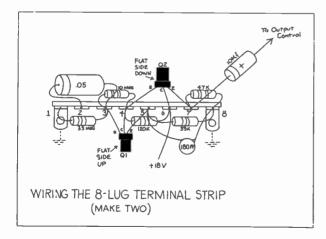
Fig. 2—How to wire the 8-lug terminal strips that support the amplifier modules. Be sure the plus sign on the 10-µf capacitor is toward the strip, not toward the output control.
