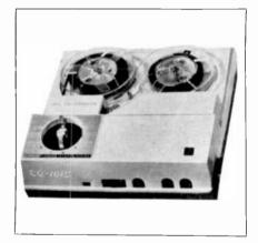
To outward appearances, this machine is very ordinary; it looks more or less like most Japanese transistor recorders. But the similarity ends there. This compact two-hands full has a positive capstan drive and two speeds—35¼ and 17½ imps. The capstan is covered by a removable drum whose larger diameter provides the faster speed. Changing speeds is relatively easy,
