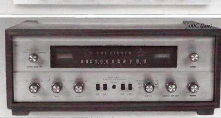
The stereo beacon used an electronic switch to eliminate pops from a relay when switching to multiplex converter. The stereo multiplex on board was a time-division type and consisted of two balanced four-diode bridges and a 38 kc synchronous oscillator, which acted as an electronic switch. Some Fisher enthusiasts prefer the sound of the 500B to the 500C because of the non-Nuvistor front end. They opinion is that the Nuvistor circuit is less open sounding.
