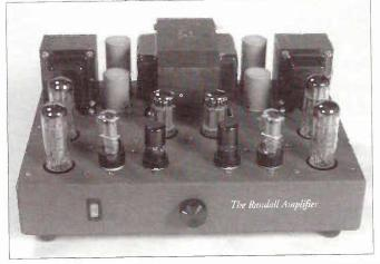
solid chassis. Anyone using a tube amplifier has already foregone lightness and efficiency, so we might as well go all the way. Besides, steel is cheap. A grey-wrinkle powder coat finish is used. This is remarkably like the classic solvent-based wrinkle finishes, but is very rugged and environmentally-friendly. Drawings were made up, and the chassis were built by a local sheet-metal shop, U.S. Fabrications, in San Jose, California.
