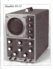
As mentioned earlier, a triggered sweep is recommended. An enhancement to the triggered sweep is the delayed sweep, which permits the sweep to start after an adjustable delay time. This is not too useful for audio testing, but can be helpful in digital debugging.
