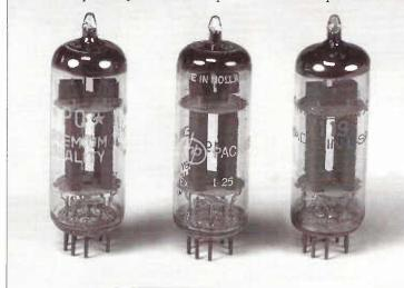
structure and a gm =  $15,500 \mu$ mhos at 36 ma. This type was brought into America as the 7119 by Amperex. Some later military 7119s were built here.
