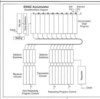
decade modules, one PM-and-clear module, one repeater module, eight pulse transceivers, two program-pulse receivers, and one gate module, all adding up to more than 500 tubes. Gating is done with 6SJ7s or 6SA7s, with their various grids receiving various pulse signals. The many gating functions require many interface arrangements, since various tubes and grids within tubes are used, all of different sensitivities.
