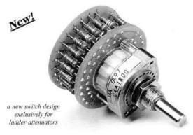
*Mono* - 1 deck, 24 position (shown) ------ \$137. *Stereo* - 2 decks, 24 position ------ \$252. off-the-shelf values: 600 ohm, 10K, 25K, 50K, 100K, 250K
