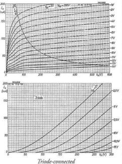
MOST GUITAR OR HI-FI AMPS. Do not attempt to use it unless you are certain that the screen voltage is 200v or less. One interesting discovery was that the SV83 was much more sensitive than any of the EL84s tested. So, if properly operated, it has great potential for new applications in guitar or hi-fi amplifiers.
