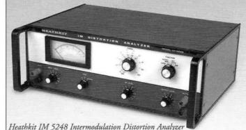
Non-linearity will cause the two signals to modulate each other, producing a series of sum and difference frequencies. The intermodulation distortion analyzer generates two frequencies, passes both through the system under test, then filters out one or both of these frequencies. If intermodulation occurs, it will generate frequencies outside of the filtered-out frequencies, which are then measured by an ÂC voltmeter.
