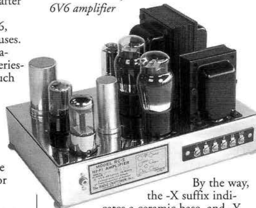
1948 RadioCraftsmen RC-2 10 watt 6V6 amplifier
