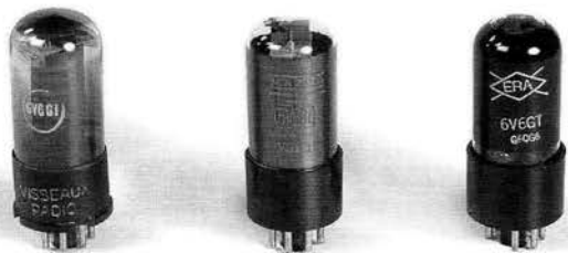
Visseaux 6V6GT (1950s), Mazda 6V6GT (1950s) and Russian 6V6GT (1990s)
