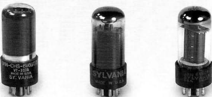
Sylvania types: JAN 6V6GT (1940s), 6V6GT (1950s) and JAN 6V6GT (1980s)
