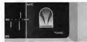
Precision-ray tuning eye makes it simple to tune precisely on both AM and FM.
