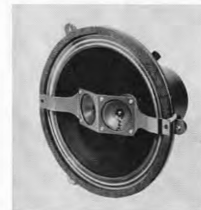
The Wigo Model CX 212B represents an economical approach to quality loudspeaker design. An extended-range single cone speaker is the basic unit, equipped with a rigid cast-aluminum frame, a very heavy magnet, and soft cone suspension. The dual tweeters are optional or can be added later if greater treble range and dispersion are desired.
