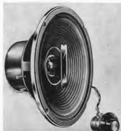
This Electro-Voice coaxial speaker employs a separate horn tweeter for extreme highs, surrounded by a mid-range cone mechanically crossed-over to the large woofer cone.
