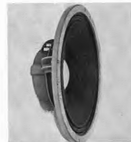
The James Lansing Model D123 is a high-quality single-cone wide-range speaker. Treble radiates from the light aluminum dome at center. Shallow depth is an advantage where space is tight.
