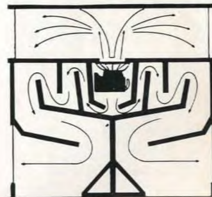
(Left)—Section drawing through a folded corner horn enclosure shows interior sound paths for highs, middle, and lows. Note the complex interior panels forming a gradually expanding horn for the bass frequencies. This design by audio engineer Stewart Hegeman serves as the basis of several Brociner enclosures.
