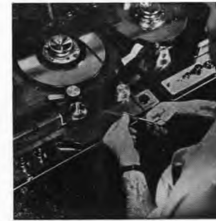
Editing magnetic tape is as easy—even easier—than editing movie film. Scissors and splicing tape do the job.
