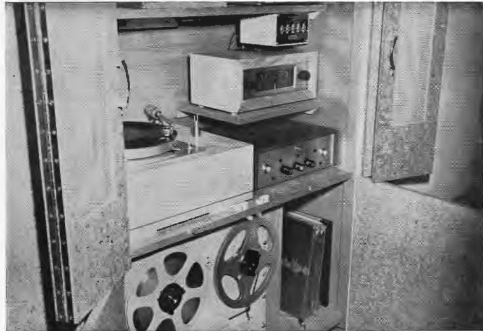
A closeup view identifies the tuner as a Fisher, the amplifier as a Scott, the turntable as a Metzner with a Rek-O-Kut arm (bearing a Pickering cartridge), and a Revere tape machine. The small box atop the tuner is Mr. Cadarette's own switching arrangement that eliminates a lot of unsightly wiring.
