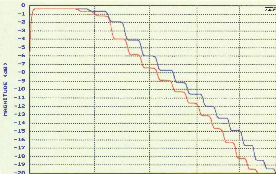
FIGURE 1: Matching between channels of stepped input attenuation, first 20 dB shown.
