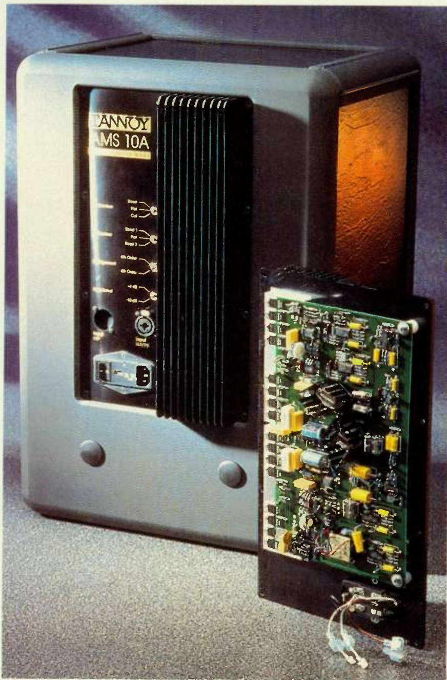
KEEP ITS COOL: The heat-sink fins on the rear of the unit keep the AMS-10A's from showing stress.
