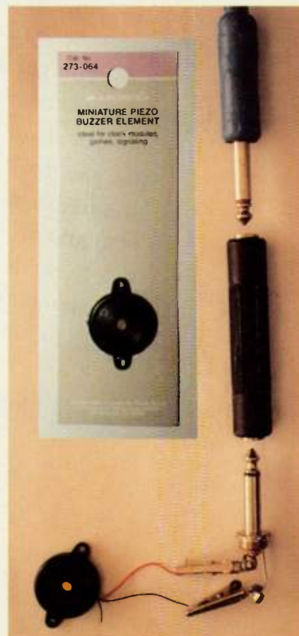
IT FIGURES, PART 1: Fig. 1 (inset, right) shows the Piezo package. Fig. 2 (right) illustrates the proper hook-up. Fig. 3 (above) shows how the Piezo should be attached to the drum head.
