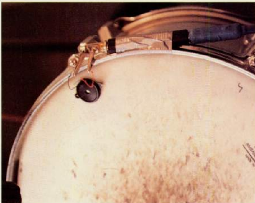
IT FIGURES, PART 1: Fig. 1 (inset, right) shows the Piezo package. Fig. 2 (right) illustrates the proper hook-up. Fig. 3 (above) shows how the Piezo should be attached to the drum head.
