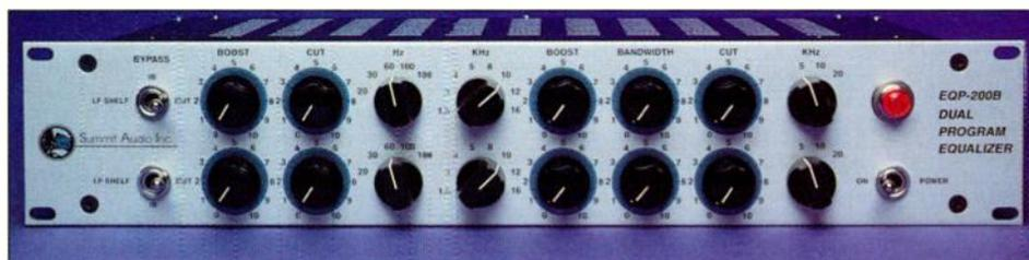
**O**ffering a selectable low-frequency 6-dB-per-octave shelving filter starting at 50 Hz, Summit Audio's EQP-200B dual-program EQ builds on the design of the EQP-200A. The low-frequency boost/cut section is enhanced with the addition of 180 Hz to the existing frequencies of 20, 30, 60,
