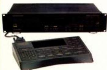
Both next-generation stand-alone write-once CD recorders, the CDR615 & 620 offer built-in sample rate conversion, CD/DAT/MD/DCC sub-code conversion, and adjustable dB level sensing. Additional features include adjustable fade in/fade out, record mute time, & analog level automatic track incrementing. A 9-pin parallel (GPI) port and headphone output with level control are also included.
