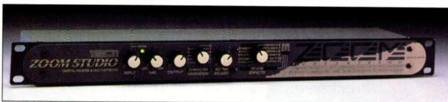
banks x 11 variations — which are instantly available at the user's fingertips. The unit's specifications include 44.1 kHz sampling and 18-bit A/D and D/A converters and full stereo implementation. For more information, contact Samson Technologies Corp., P.O. Box 9031, Syosset, NY 11791-9031. Tel: 516-364-2244. Web: [www.samsontech.com](http://www.samsontech.com). Circle EQ free lit. #104.
