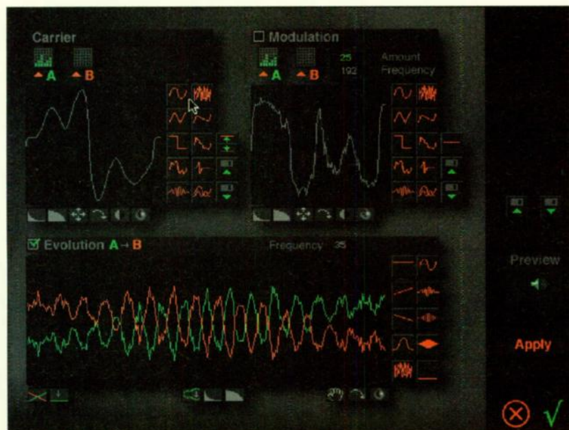
FIGURE 5: The Procedural Synth creates a sound via frequency modulation synthesis, where a sound, or "carrier," is mathematically modified by a second waveform, or "modulator."
