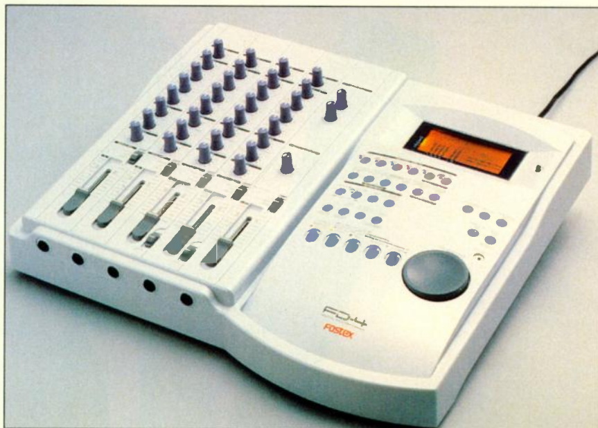
FANTASTIC 4: The Fostex FD-4 is a standalone hard-disk recorder.
