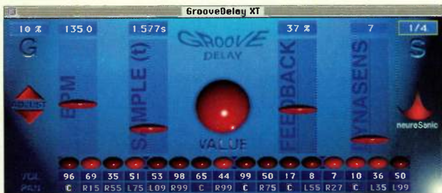
FIGURE 2: The Groove Delay is a digital tapped delay optimized for adding rhythmically related echoes to dance grooves.
