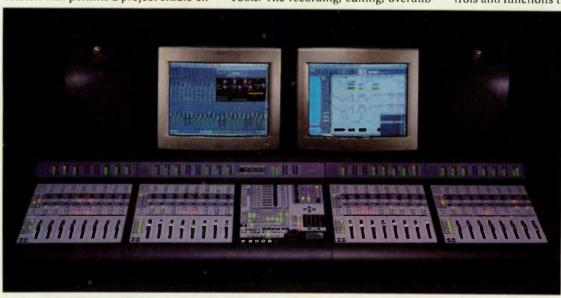
TOTAL CONTROL: ProControl can be expanded up to a total of 32 faders.
