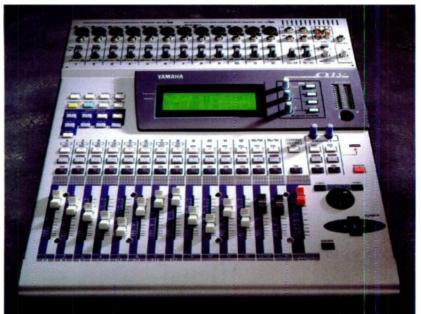
smooth-touch motorized faders. But it's the memory capabilities of the 01V that allow you to create your best mixes. Snapshot memory of all mixer settings allows you to store your mix settings with the simple press of a button, so you can come back to the mix at any time. Useful "libraries" allow you to store your favorite settings for EQ, Effects, and Dynamics. These can be recalled at any time and applied to any mix, so you can use that perfect sound you had the last time.
