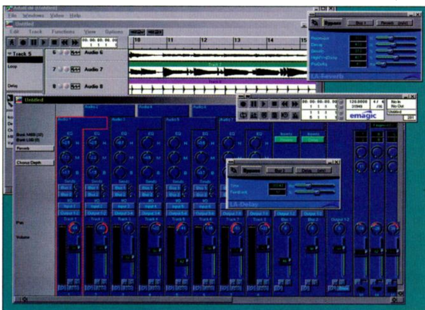
FIGURE 1: Emagic's ADAT Edit software, part of the Alesis ADAT Edit package, essentially treats ADAT as a removable storage medium. It transfers audio files to disk, which you can then edit, cut, mix, process, etc., and run in parallel with MIDI tracks.
