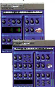
Both Bruno and Reso create rich, unique sonic textures using new cross-synthesis techniques to "synthesize" existing audio in real time. Specifically, Bruno uses time-slicing, a technique whereby timbres are extracted from the source audio during playback and crossfaded together, and Reso (as the name implies) uses a resonance generator to add harmonic overtones to audio.
