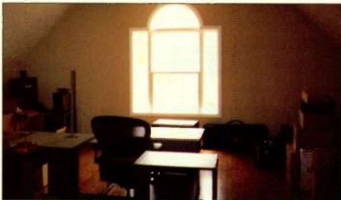
This is how our room looked before we began installing acoustic materials. The walls and ceiling are all hard surfaces, the floor is hardwood. As you'd expect, the room was bright sounding and had a very long reverb time with prominent slap echoes.
