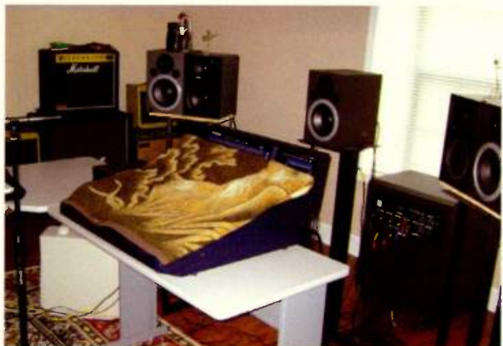
Here's how the Audio Precision System acoustic tests were set up, in this case before the room had been acoustically treated. An Earthworks mic was fed into the A-P analyzer; the blanket on the console is to cut down on reflections. Careful measurements were taken so that the test could be accurately duplicated after the room had been treated.
