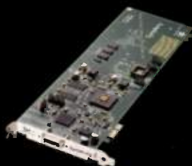
Symphony PCI E Card 32-Channels of I/O per card & up to 96 channels per system
