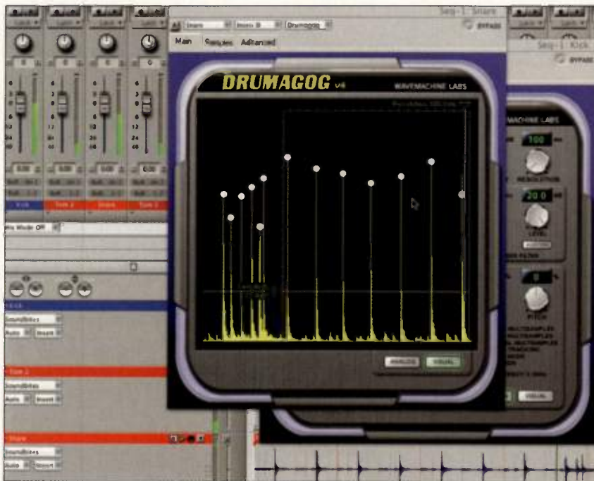
Fig. 2: Two instances of Drumagog are inserted in Digital Performer; one is replacing the snare hit, and the other, the kick. The front instance is running in Visual mode, which makes it easy to set the sensitivity and resolution for optimal triggering.
