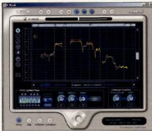
Fig. 1: Sonar's V-Vocal can do automatic pitch correction, add or subtract vibrato, and control dynamics of vocal (and other mono) tracks in real time — but it can also change timing and "groove."
