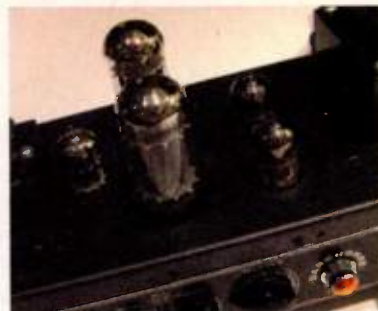
Traynor's DarkHorse features an all-tube design.
